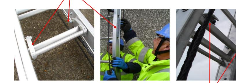
Make sure the latch locks and rests fully on the rungs before it is erected to working height
